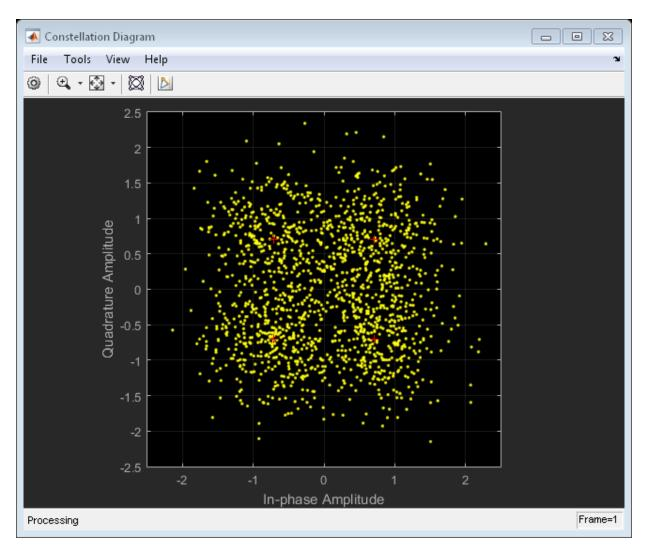
Demodulate the noisy symbols to obtain soft bits. Convolutionally decode the soft bits. Display the number of erroneous bits
